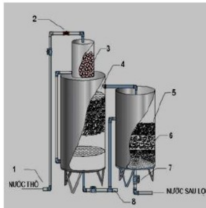
SAND FILTER TANK
